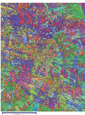
◀ Additively manufactured Ti64 alloy analysed using 20 nA beam current:
