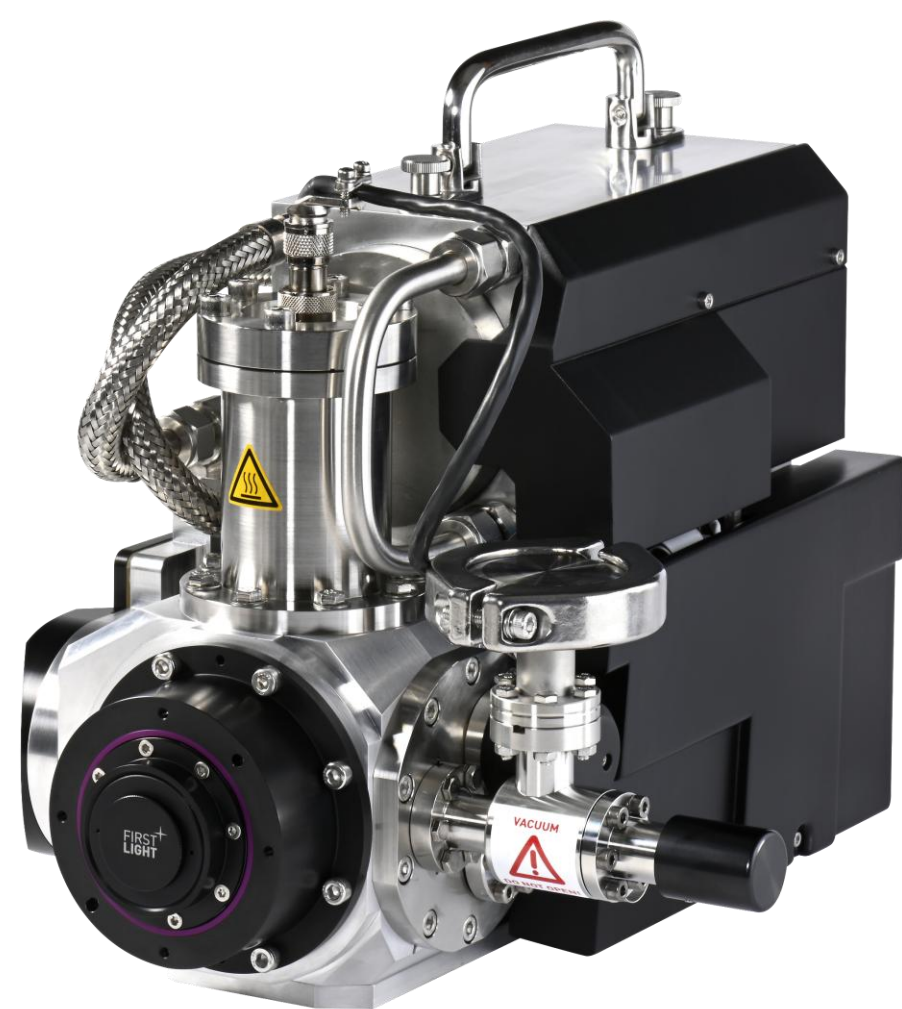
Figure 1 - C-RED One (right) is a high-speed electron-multiplied infrared camera fabricated and commercialised by Oxford Instruments First Light Imaging. It offers world-leading single photon sensitivity and rapid non-destructive readout at 1000s of frames/s. Details on C-RED One's Saphira sensor are outlined below. C-RED One is an autonomous user-friendly plug-and-play system that can be operated in remote locations. The sensor is enclosed in a self-managing vacuum chamber and is cooled to <90 K with an integrated cryogen-free pulse tube cooling system. The camera is described extensively by Feautrier et al. [5]. Learn more about C-RED One by scanning the QR code on the left.
