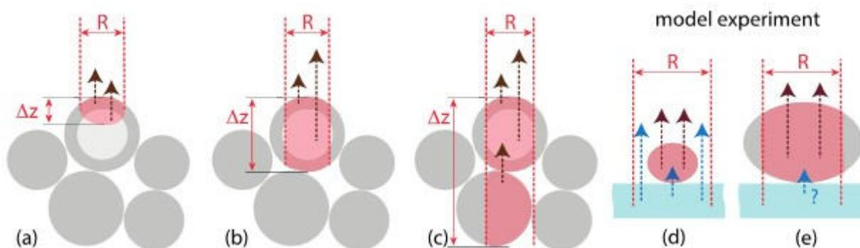
A schematic illustration of possible μRS probing depths for a micro-scale powder system (a)-(c) and a single particle on RS-active substrate (d) and (e).
