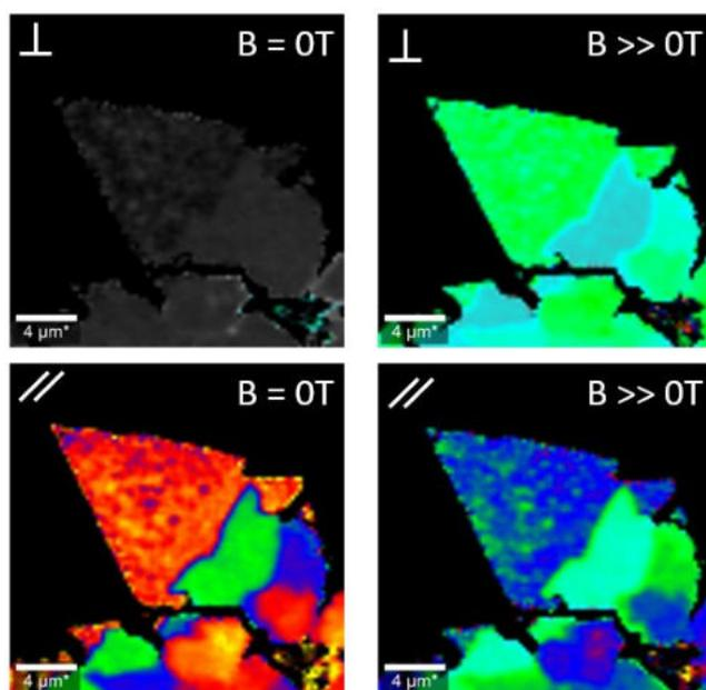
Intensity ratio of two characteristic Raman signals of MoS<sub>2</sub> recorded at 2K for different magnetic field strengths and polarization states
